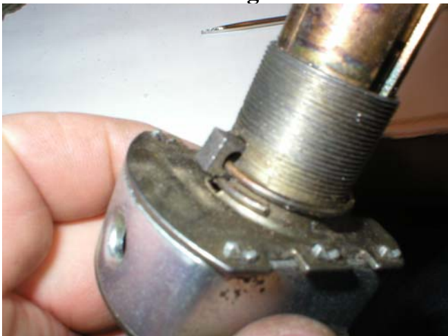
Lock Case is staked together
