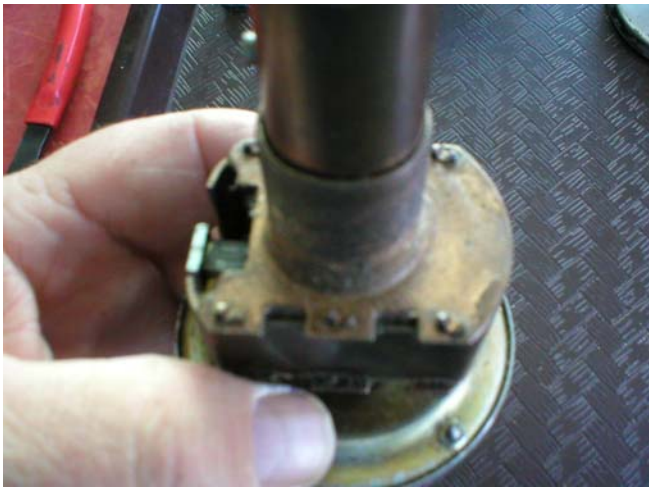
Lock Case is staked together
