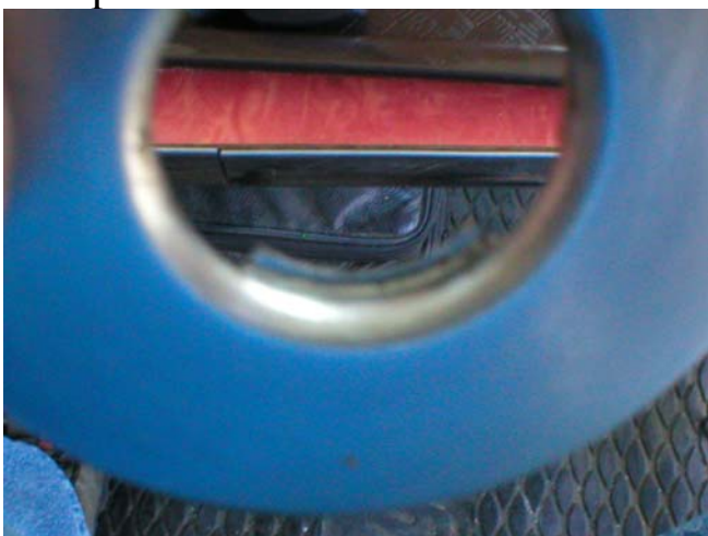
Faceplate flange that fits into the cylinder itself.
