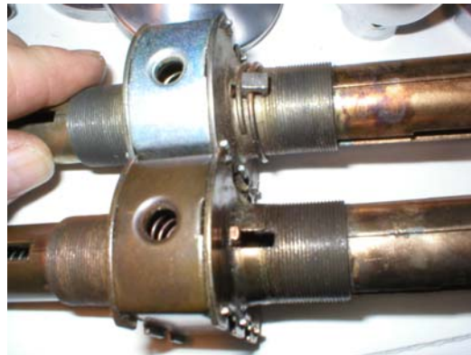
Entry & Storeroom lock cases notice the locking tabs
