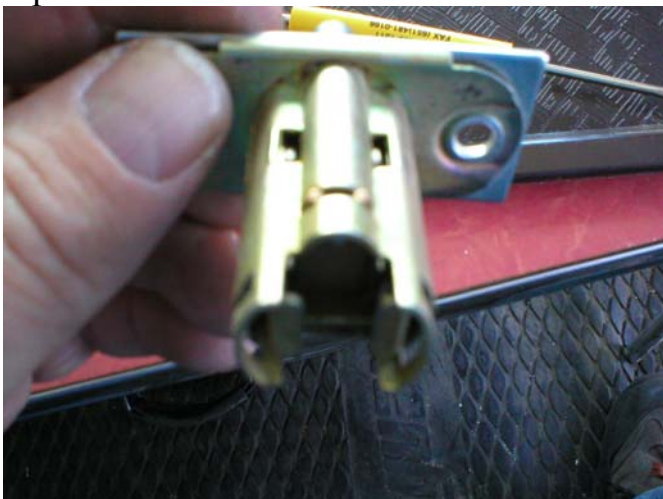
Back of Latch at rest
