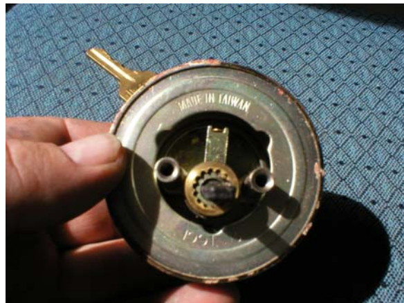
Backside of case, cylinder will slip out of outer shell
